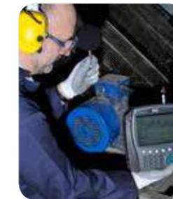
The Microlog Analyzer range includes route-based instruments that work with powerful SKF predictive maintenance software systems and stand-alone instruments that offer on-the-spot advice and signal analysis capabilities. Both options enable you to migrate from time-based to condition-based maintenance, helping you to reduce the risk of unplanned
